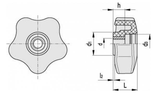
$\begin{array}{lll} D & = 63 \\ d1 & = 22.5 \\ d3 & = 19.5 \\ dh & = 12 \\ h & = 15 \\ I2 & = 1.3 \\ L & = 21.5 \\ Weight in (g) = 34 \end{array}$
